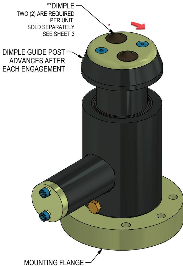
PROTECTS DIES BY MINIMIZING POTENTIAL FOR MULTIPLE BLANK FEEDS
