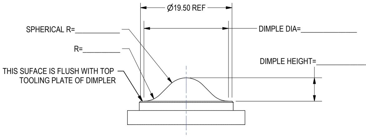
THIS WORKSHEET IS FOR THE MANUFACTURING OF WELKER CUSTOM DIMPLES (TO BE USED WITH WELKER WD3 DIMPLER).
